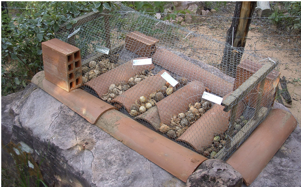
Fig. 4. The wire-mesh enclosure where nuts and shells have been kept to reveal the effect of natural weathering.
