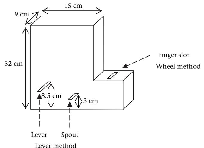
**Figure 2.** Foraging apparatus: juice dispenser with two methods of solution, lever method and wheel method.
